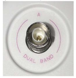
The remaining dual-band RP-TNC ports that do not support Self-Identifying Antennas can be differentiated by the standard orange color text around the connector. Self-Identifying Antennas can be used on any of the RP-TNC ports of the AP. However, only port A will read the antenna as a Self-Identifying Antenna.
