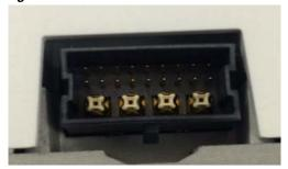
Figure 12 AIR-CAB002-DART-R= DART Connector
