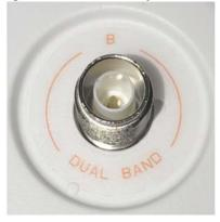
When the 9120AXE or 9120AXP AP is powered up with a Self-Identifying Antenna connected to it, the AP's circuitry reads the EEPROM in the Self-Identifying Antenna. This enables the AP to automatically configure the antenna gain and beam-width. However, if supported legacy antennas (see "List of External Antennas Supported on C9120AXE and C9120AXP") are used with this AP, the antenna parameters must be manually configured in the wireless controller as with older APs.
