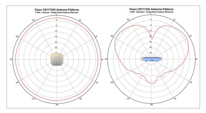
**Figure 1.** Antenna radiation patterns for the 9117I
