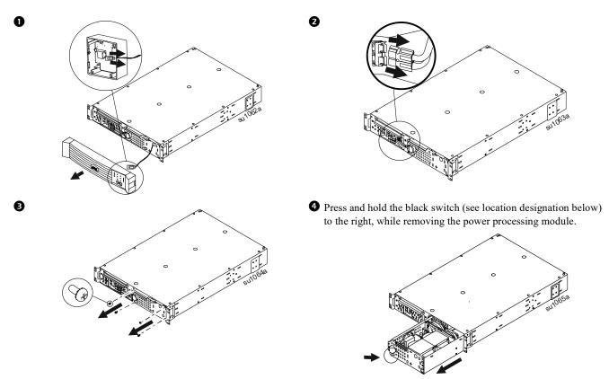
**Note**: Reverse steps 1-4 for installation of the new module.
