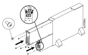
**5** Snap the display bezel out through the rear to rotate the bezel.
